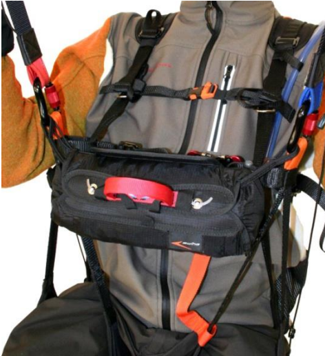
Positioning the Brave 4 front container
