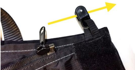
Direction to install the speed bar line through the pulleys
