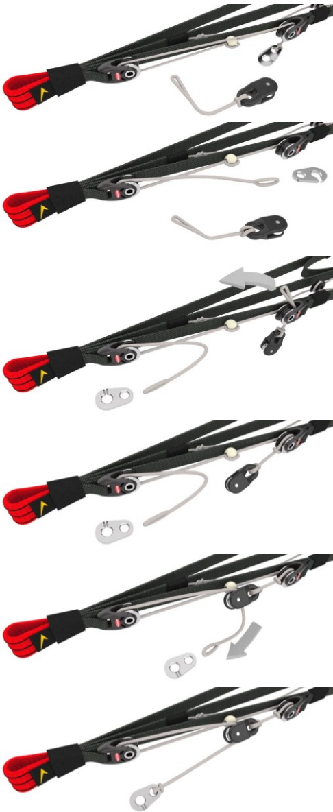
Fig. 9 Installing the speedlimiter
